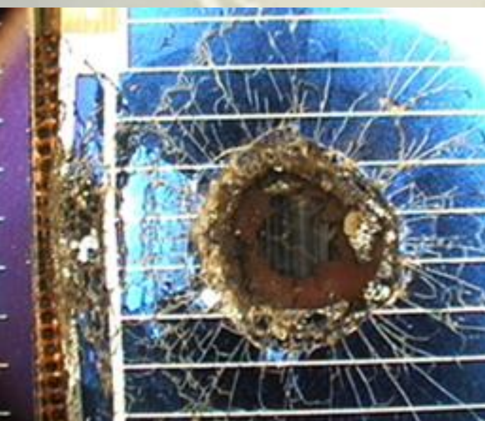
Solar cell damage, caused by impact
