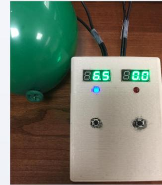
Figure 4, The assembled device in 3D-printed chassis. The device is detecting negative charges by rubbing a balloon on hair (blue LED indicator, 6.5 Volt)
