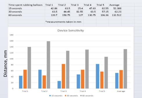
Figure 5, Device sensitivity test (Effect of time and distance on detection of electrostatic charges)
