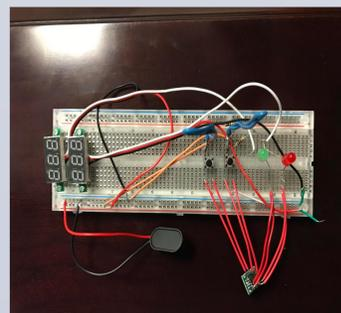
Figure 3, A photo showing the main components of the circuit including voltmeter, reset buttons, and LED indicators (for +ve and -ve charges)
