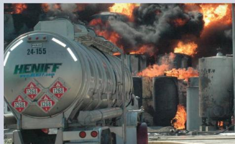
Figure 1, Static Spark Ignites Explosion Inside Flammable Liquid Storage Tank (source: Internet, CSB: Barton Solvents Case Study)
