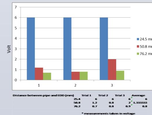
Figure 6, Device sensitivity test for polyethylene pipe
