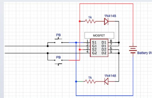
Figure 1, Circuit Diagram showing MOSFET Integrated Chip used in the design
