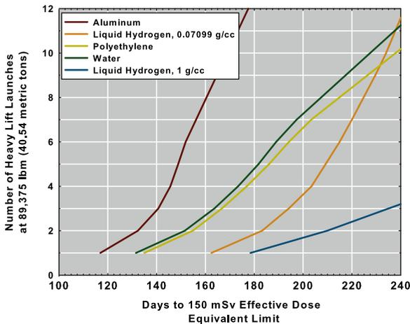
**Fig. 7.** The number of days to the 150 mSv exposure per mission for various shielding materials (inset).
