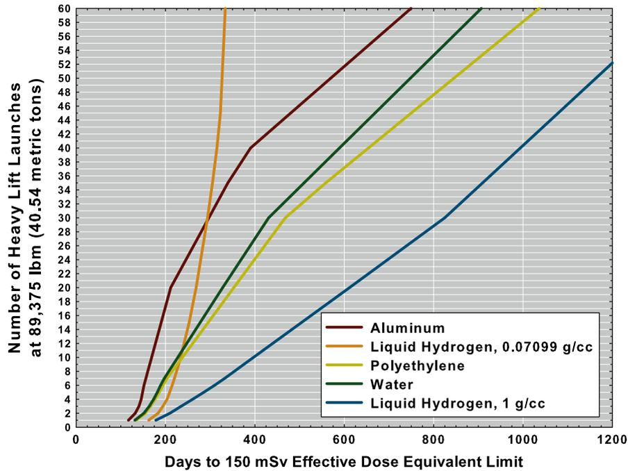
**Fig. 6.** The number of days to the 150 mSv exposure per mission for various shielding materials. (For interpretation of the references to color in this figure legend, the reader is referred to the web version of this article.)
