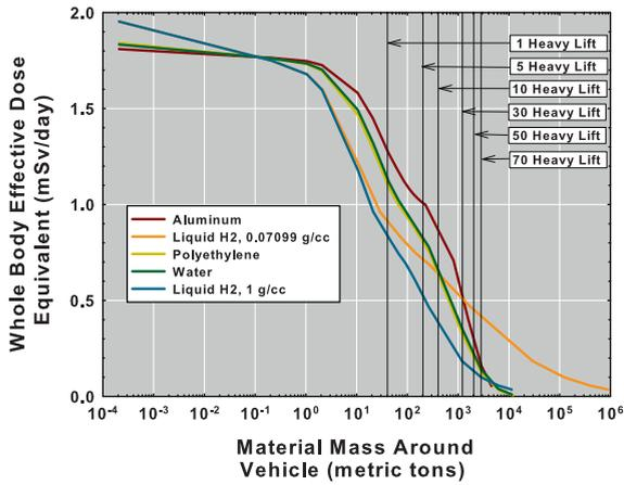
**Fig. 3.** Whole body effective dose equivalent in mSv/day for a shielding material in a spherical vehicle. (For interpretation of the references to color in this figure legend, the reader is referred to the web version of this article.)
