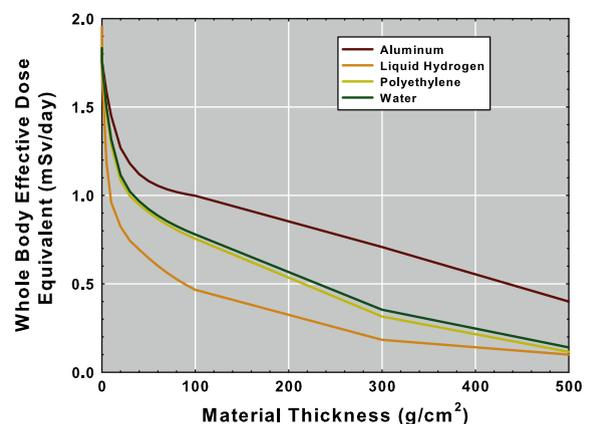
Fig. 2. Standard whole body effective dose equivalent in mSv/day to the thickness of a material in  $\text{g}/\text{cm}^2$ .
