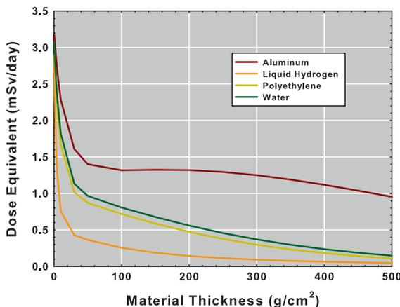
Fig. 1. Standard dose equivalent in mSv/day to the thickness of a material in  $\text{g}/\text{cm}^2$ .
