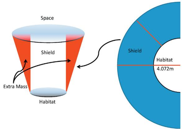
**Fig. 4.** Geometry of vehicle showing extra mass carried by the geometry. (For interpretation of the references to color in this figure legend, the reader is referred to the web version of this article.)
