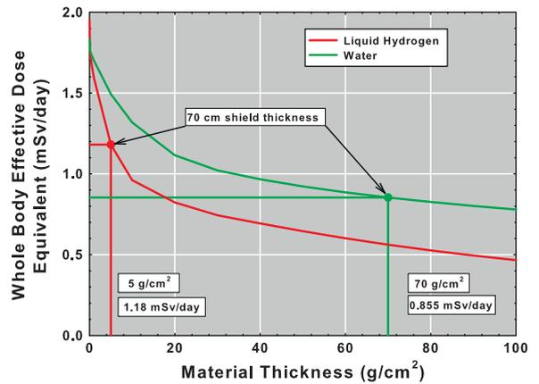
**Fig. 5.** Example of liquid hydrogen and water from Fig. 2 in a spherical shield at a constant thickness of 70 cm.
