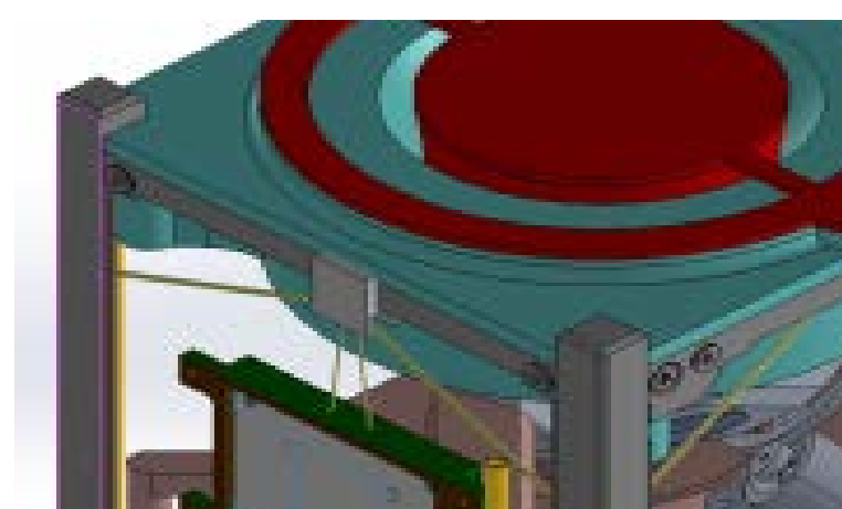
Original Design Sun Tracker New Design The sun tracker, as its name implies, will track the motion of the sun when it is deployed from the CubeSat.
